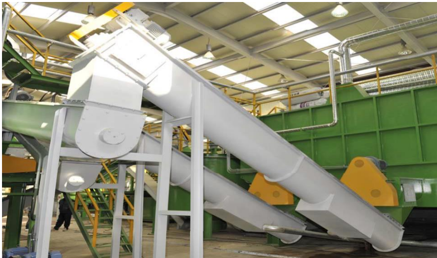
■ Screw conveyor (Order production)
